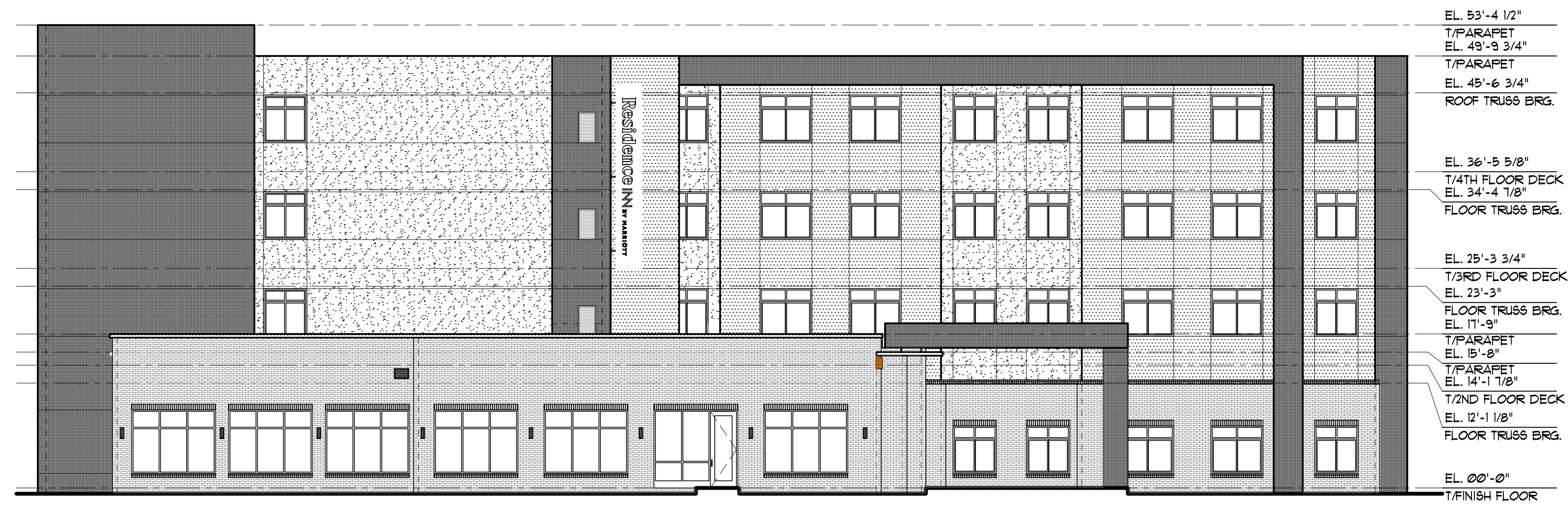
2 SOUTH ELEVATION SCALE: 3/32" = 1'-0"
