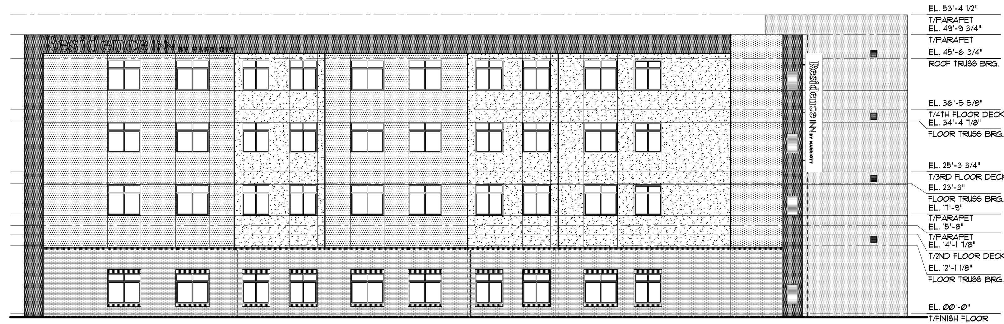
1 NORTH ELEVATION SCALE: 3/32" = 1'-0"
