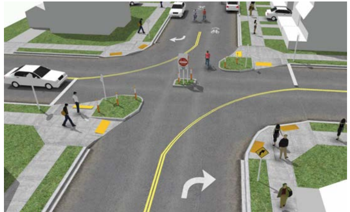
Intersection Right Only Diverter. Source: NACTO
