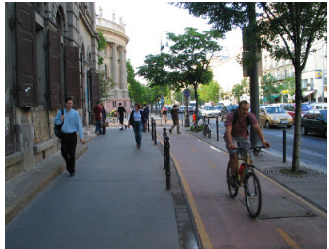
Two Way Cycle Track - Bike lanes are separated from sidewalks. Photo Credit: People for Bikes
