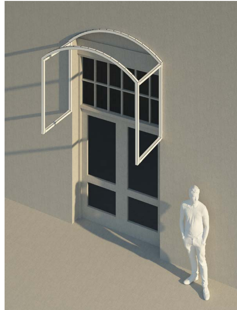
2" BLACK TUBE STEEL ROOF SUPPORT
