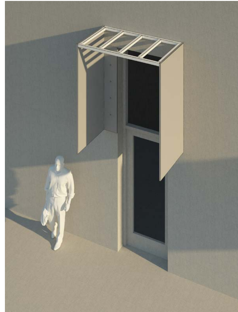
2" BLACK TUBE STEEL ROOF SUPPORT
