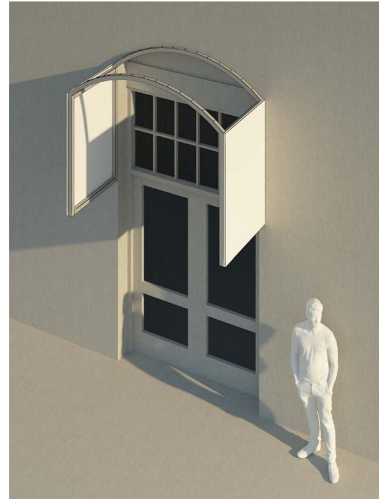
BLACK RAW STEEL PANELS FASTEN TO TUBE STEEL SUPPORT 3'-0" DEPTH FROM WALL GAUGE TBD PER FABRICATOR
