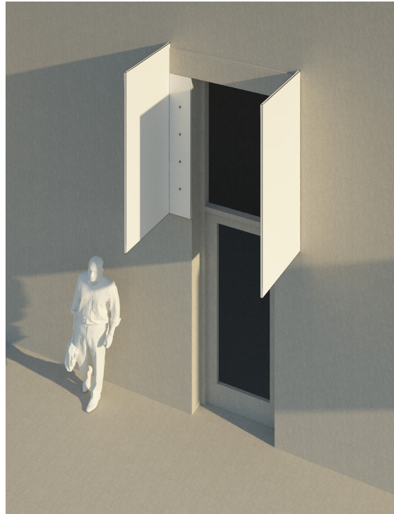
BLACK RAW STEEL - CUT AND BENT EXPOSE EXISTING CONCRETE SILL EXPOSED FASTENERS INTO BRICK 3'-0" DEPTH FROM WALL GAUGE TBD PER FABRICATOR
